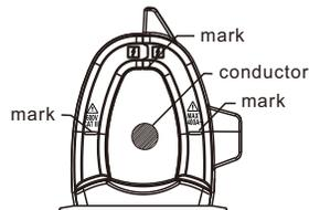
For AC current measurement, keep the conductor in the center of the clamp; otherwise the reading can deviate as much as 1.5% of actual measurement.
