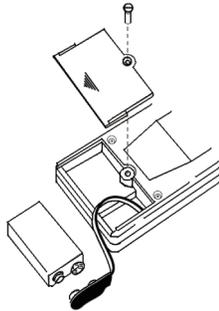
**Figure 4. Battery Replacement**
