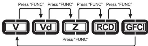
**Voltage (V):** real time display of TRMS of phase voltage, wiring status and frequency. This test item includes 3 submenus, namely phase voltage (L\_N) TRMS, voltage to earth of neutral line (zero line) (N\_E) TRMS, peak voltage (Peak). Press Up "▲" or Down "▼" selection key on the sub test item to enter the relevant test item.
